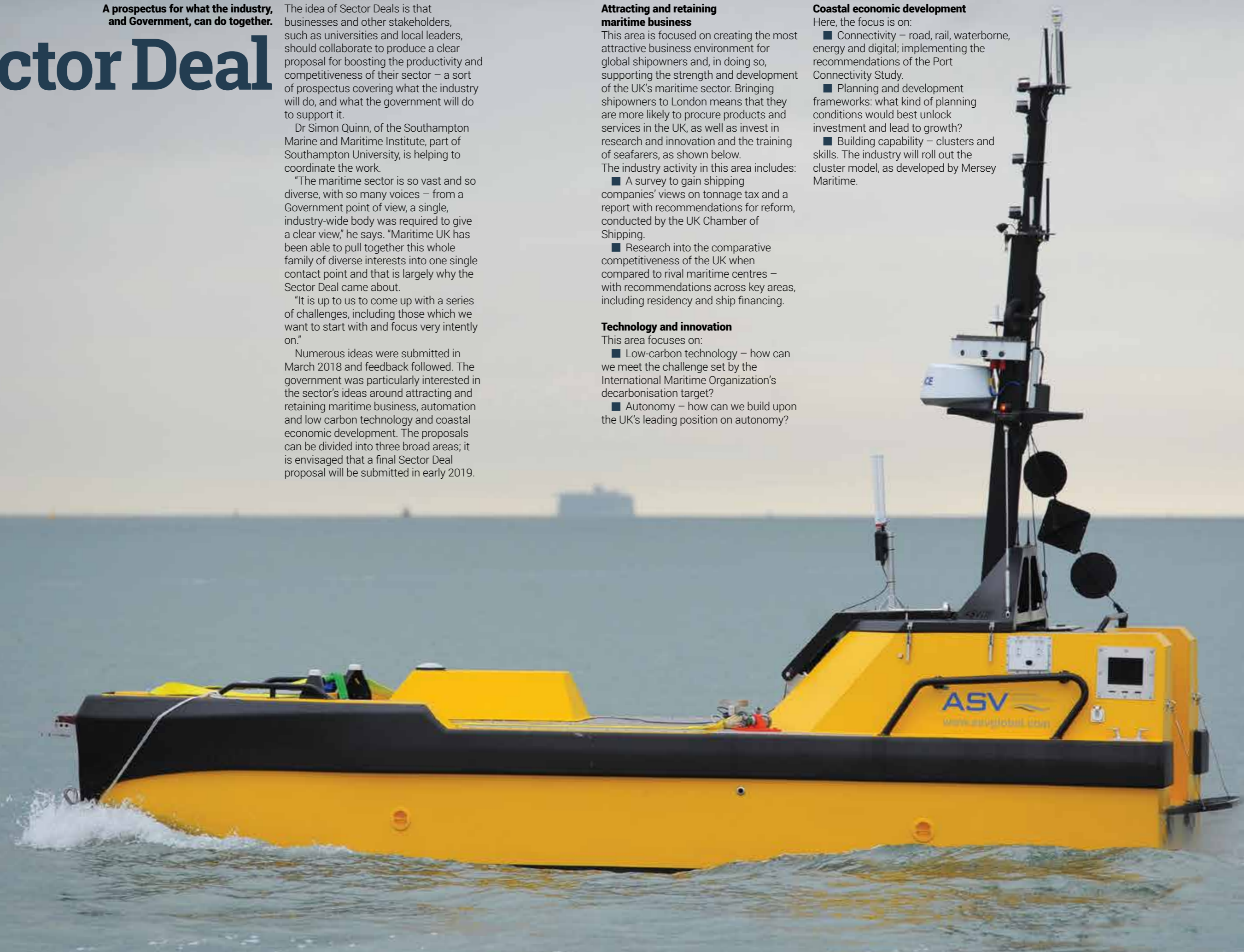
ASV Global's C-Worker 7, the UK's first fully-autonomous vessel, was admitted to the UK Ship Registry in November 2017. The 7.2 metre self-operating vessel controlled directly or remotely, can stay at sea for up to 30 days.
