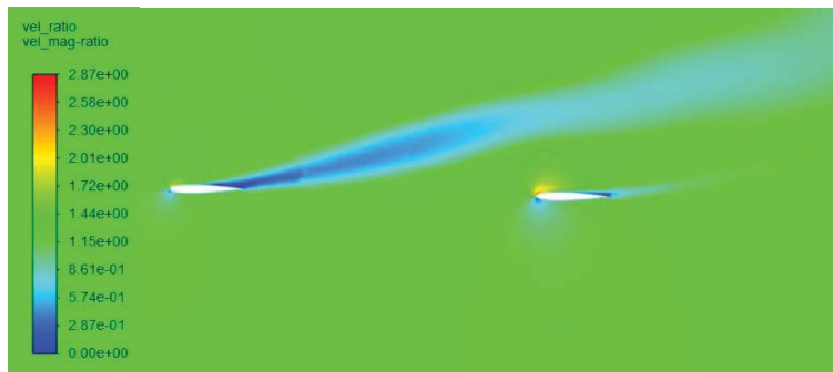
Fig. 16 to 20: Contour plots velocity magnitude ratio \frac{vel_{mag}}{vel_{inlet}} ; A pitching cycle at 50% Interfoil Spacing, +/- 14 deg. prescribed pitch motion
