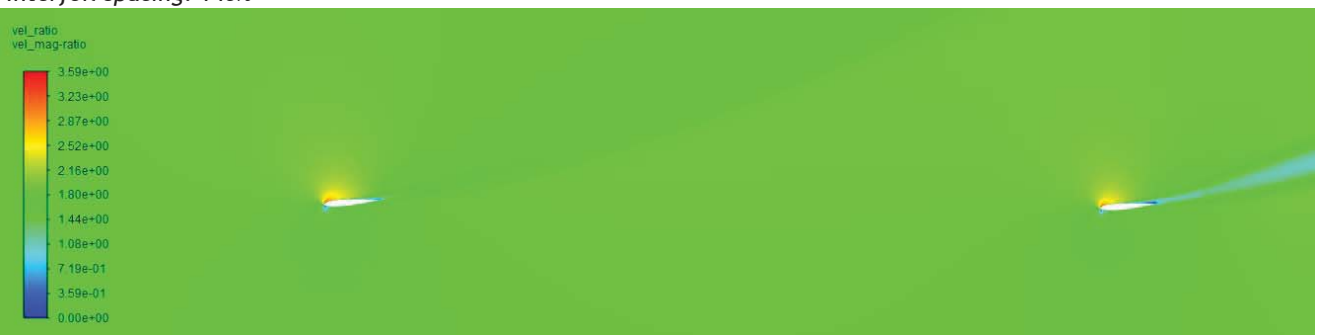
Fig. 40 to 43: Contour plots velocity magnitude ratio \frac{vel_{mag}}{vel_{inlet}} ; At maximum inlet velocity, prescribed pitch motion based on experimental data
